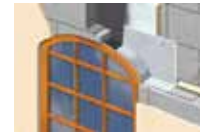
Parabolic Arch lintel
